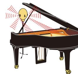
Using a microphone installed in each ear of a dummy, this recording system can capture Yamaha CFX full concert grand piano sound the way it would be heard naturally. As a result, when an SH-type SILENT Piano™ is played in silent mode, the player feels as though the digitally sampled sounds are coming directly from the piano.
